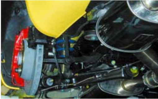
S4 with modified rear braking system
